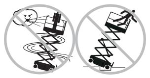
7) In the elevated state of the platform, the machine cannot run on uneven terrain, an unstable surface, or in other dangerous situations, or near these areas.
