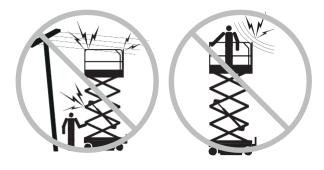
2) This machine should be kept an adequate safety distance from power line and electrical equipment according to applicable government laws and regulations and the following table.
